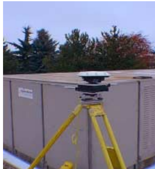
Figure 6. Station MULT showing precise translation stage and presence of heating/cooling units.
